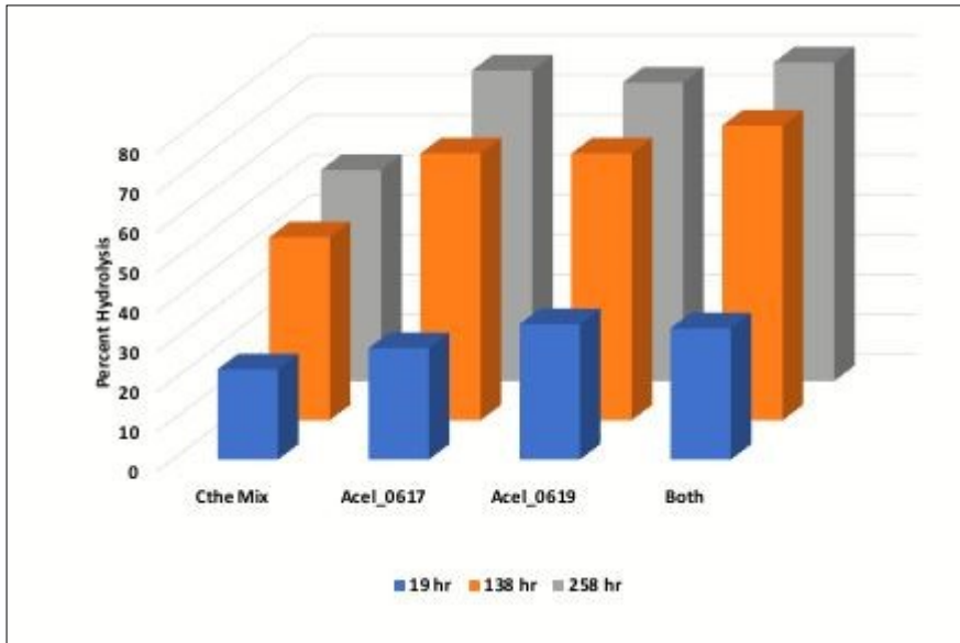
Figure 6. Hydrolysis of filter paper by Cthe enzymes supplemented with Acidothermus cellulases
